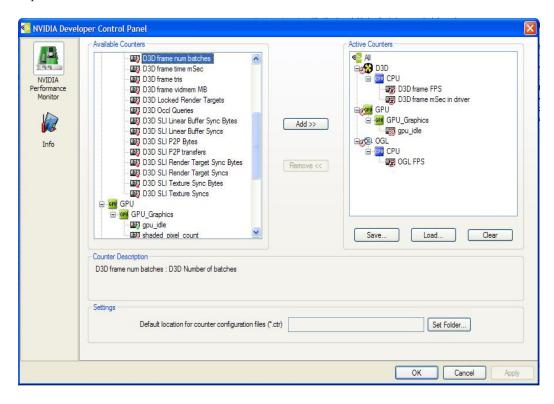
Before you try to sample a counter, make sure you have added it to the list of **Active Counters**. The GPU can sample a pre-set number of counters per clock, and this number can vary from GPU to GPU. If you choose more than this number of counters, the GPU counters are sampled in a round robin fashion, and the list on the right will show an *approximately equal* icon to reflect the reduced accuracy.
