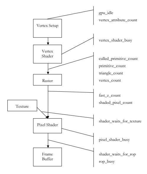
This block diagram shows where in the GPU pipeline each counter falls.
