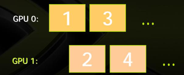
Scan-out toggles where to read framebuffer from
