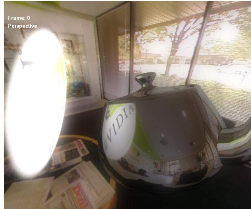
Environment-mapped background, reflected card-shaped light source, 16-bit blending with overbright bloom
